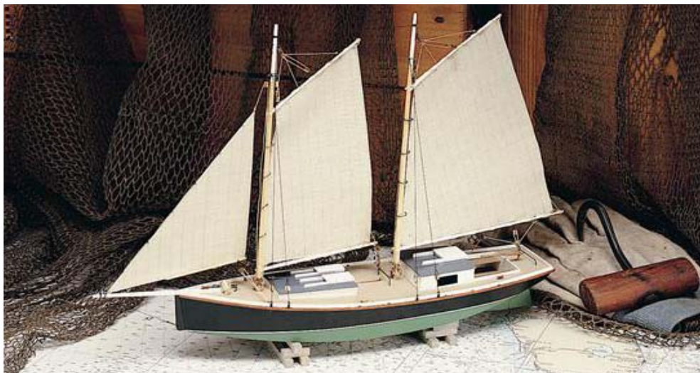
77-968 SHARPIE SCHOONER Length: 17", Beam: 3-3/4", Height: 12", Scale: (1/32), Hull Construction: Die-cut side & bottom planking
