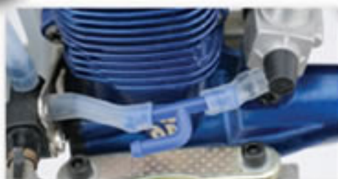
Fuel Line Open
